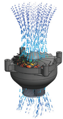
Fansink cooling performance test.
